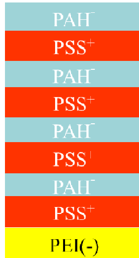
Figure 4-7: Schematic of Polyelectrolyte Layers
