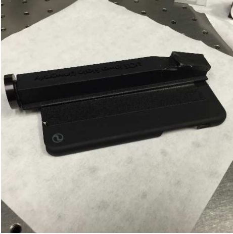
Figure 2-29: Reflectance smartphone-based spectrometer. This was used for testing and has potential to be improved further.
