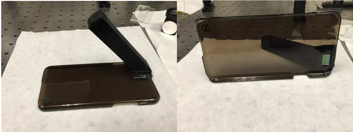
Figure 2-28: Transmission smartphone-based spectrometer. This was the final version for the transmission spectrometer made. This version provided good results but we proceeded with the reflectance spectrometer due to better results.
